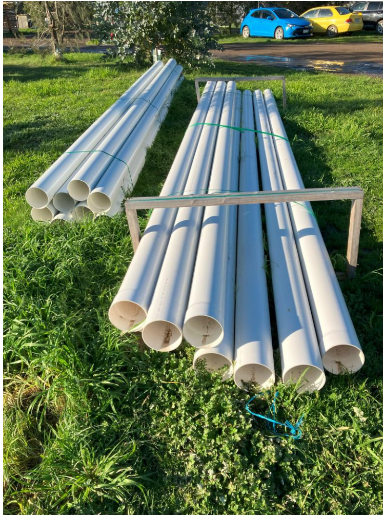
Figure 19: The pipes in this photograph are made of uPVC. It comes in fixed lengths and joins are often made with solvent welds (Photo: Pinion Advisory)
