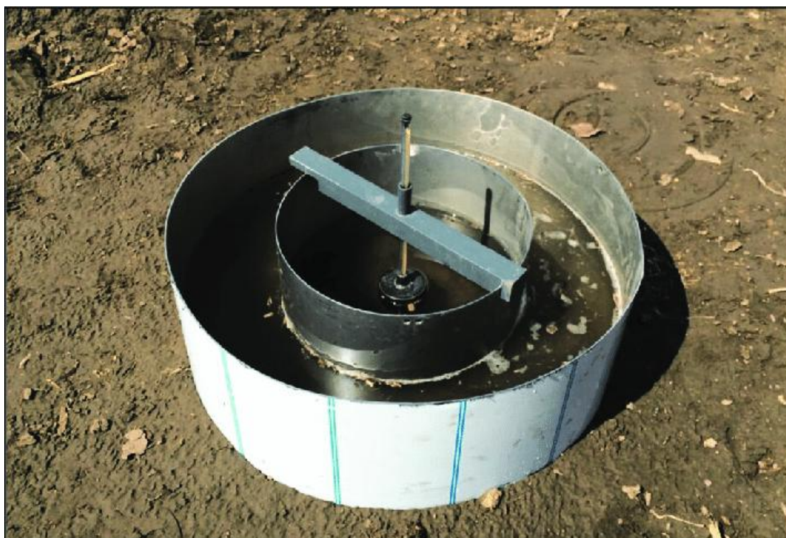
Figure 44: Infiltrometer measuring speed of water absorption into soil (Photo: (Trade India, 2025))
