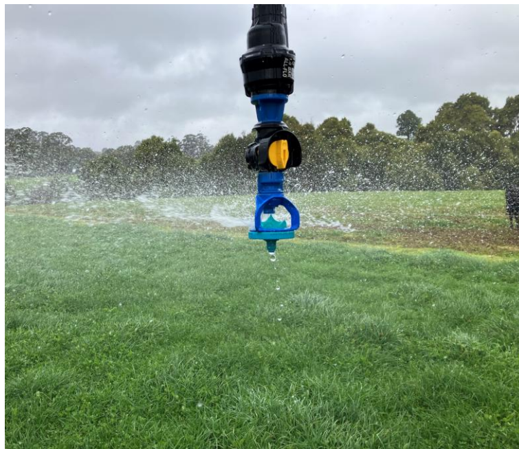
Figure 34: Low pressure sprinkler with pressure regulator for centre pivot irrigator (Photo: Pinion Advisory)
