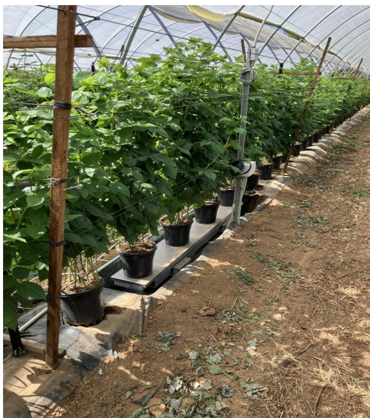
Figure 39: Lysimeters are weighing scales that contain portions of land or pots that grow crops, and are used to directly measure evapotranspiration (Photo: Pinion Advisory)
