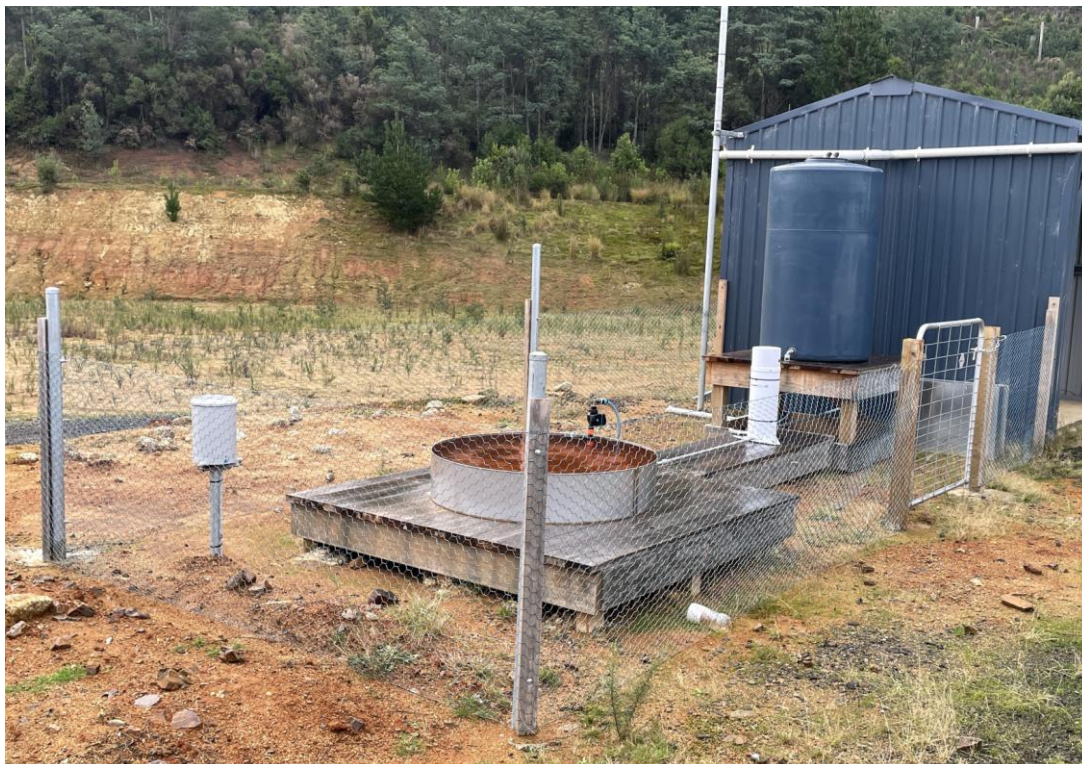
Figure 38: Class A evaporation pan, used to measure daily evaporation in a standardised manner (Photo: Pinion Advisory)
