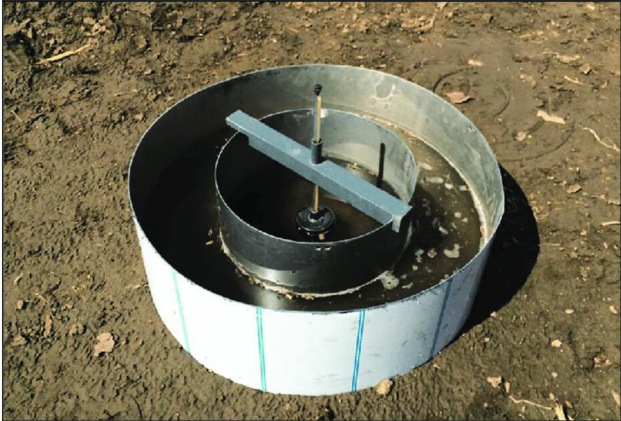
Figure 45: Infiltrometer measuring speed of water absorption into soil (Source: (Trade India, 2025))
