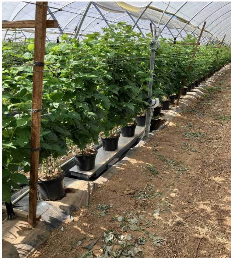
Figure 41: Lysimeters are weighing scales that contain portions of land or pots that grow crops, and are used to directly measure evapotranspiration (Photo: Pinion Advisory)
