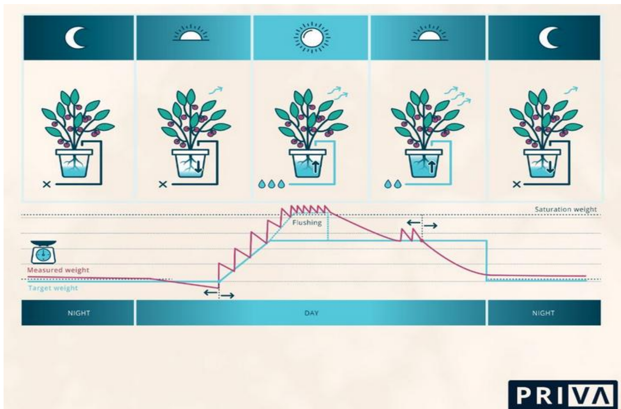
Figure 47: Substrate irrigation to match daily crop water use requirements (Source: (Priva, 2025))
