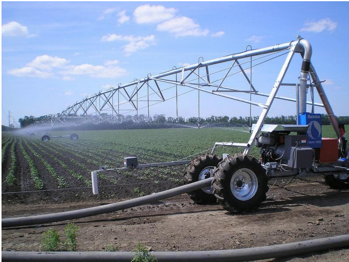
Figure 11: Hose pull linear move irrigator (Photo: (Cadman Power, 2021))
