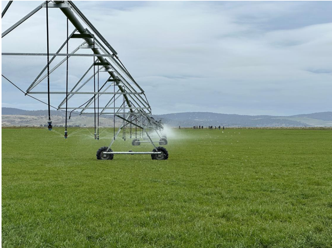
Figure 10: Centre pivot irrigator ( Photo: Pinion Advisory )
