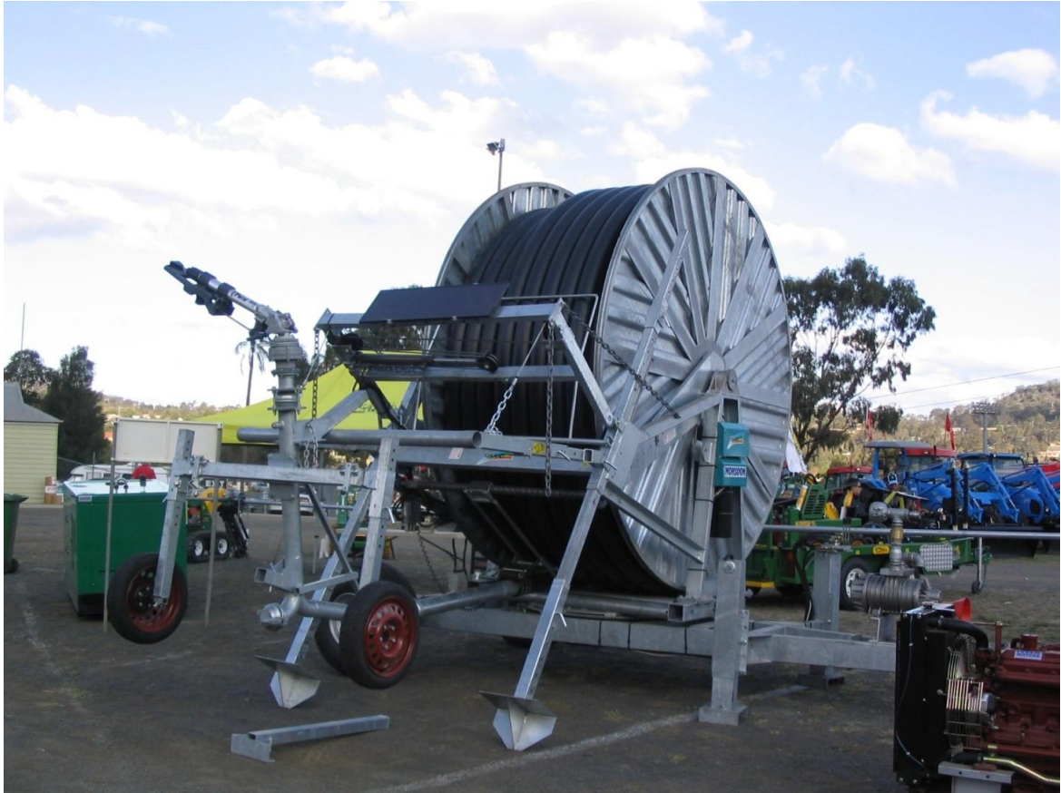
Figure 9: Hard hose travelling irrigator ( Photo: Pinion Advisory )
