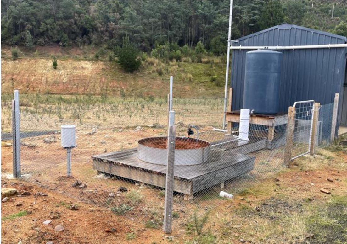
Figure 40: Class A evaporation pan, used to measure daily evaporation in a standardised manner (Photo: Pinion Advisory)
