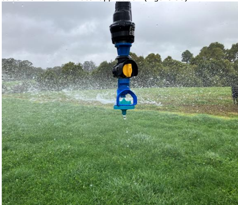
Figure 36: Low pressure sprinkler with pressure regulator for centre pivot irrigator (Photo: Pinion Advisory)
