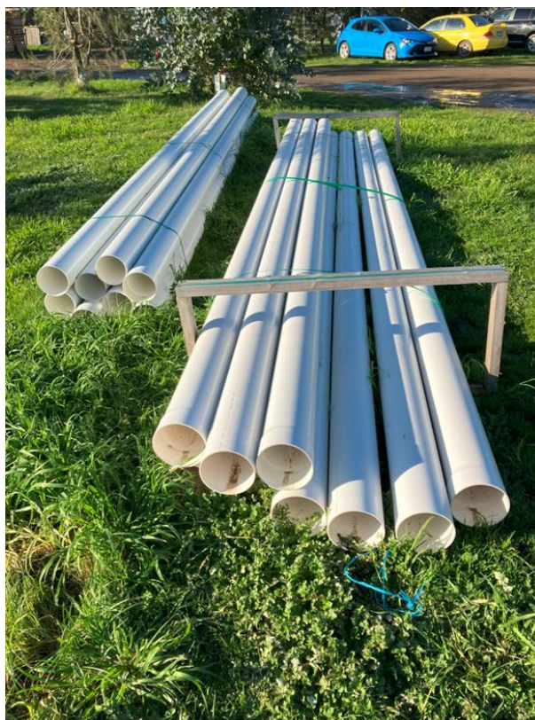
Figure 21: The pipe in this photograph is made of PVC. It comes in fixed lengths and joins are often via rubber rings or solvent welds (Photo: Pinion Advisory)
